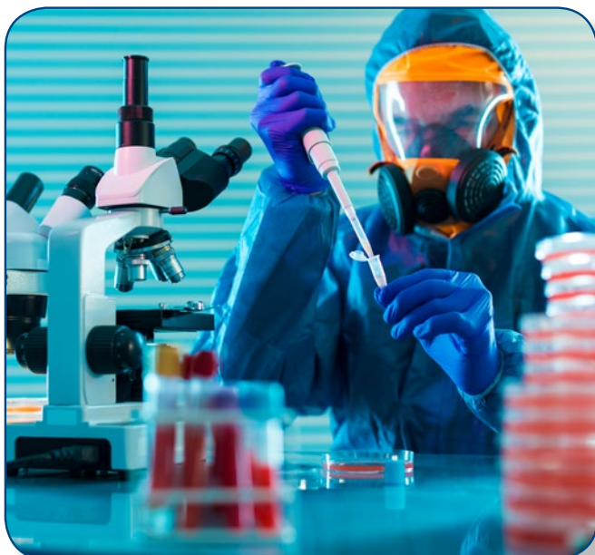
Hazmat Suit is consisting of an impermeable whole-body garment worn as protection against biohazards.
