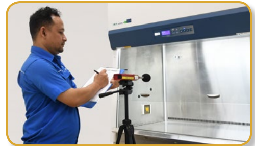
Noise Level Test
